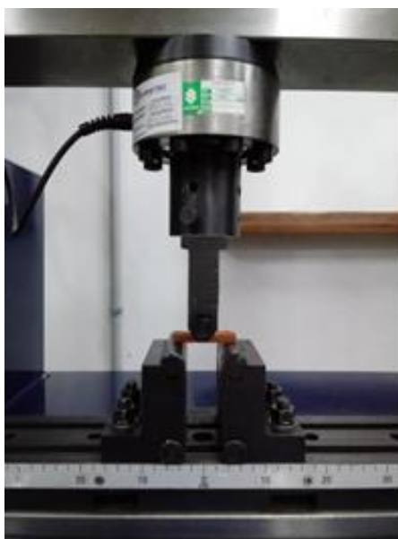
Figure 6. Flexural strength test.
