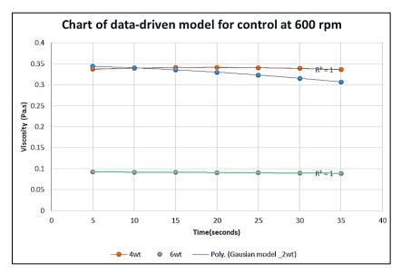
Figure 7. Chart of data-driven model for 2wt, 4wt and 6wt. % Na<sub>2</sub>CO<sub>3</sub> at 600 rpm
