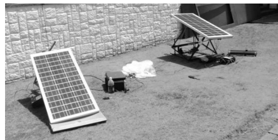
Figure 4: Testing of solar tracker with stationary tracker for comparison
