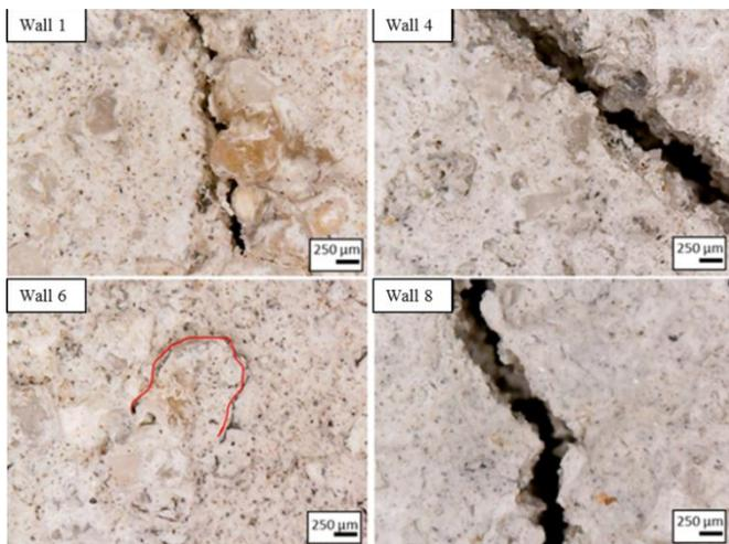
Figure 7. Fissures in the Coating
