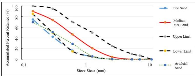
Figure 3. Gradation Curve Fine Sand, Medium Mix Sand and Artificial Sand
