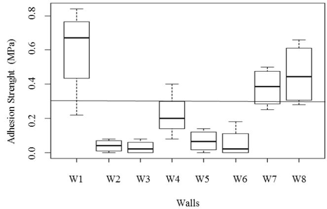
Figure 4. Adhesion results in mortar coating
