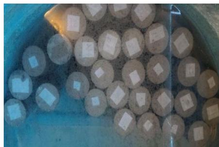
Figure 1. Submersible curing test specimens
