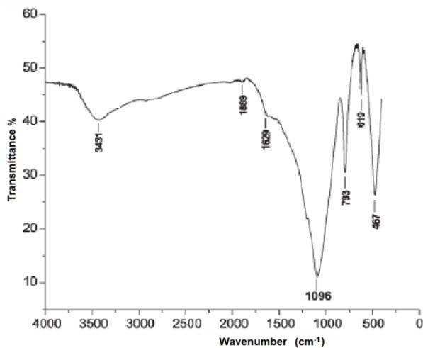
Figure 1. Infrared spectrum of an RHA sample [2].
