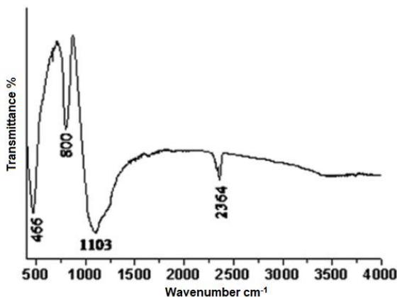
Figure 2. Infrared spectrum of an RHA sample [8].
